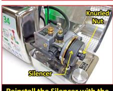
Reinstall the Silencer with the Knurled Nut. Finger tight only. Do not use tools.
