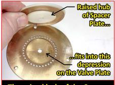
The raised hub of the Spacer Plate fits into the depression machined in the Valve Plate.
