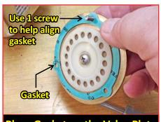
Place Gasket on the Valve Plate as shown. Use a mounting screw to help align the gasket.
